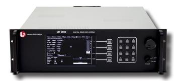
L3 Telemetry & RF Products (L3 T&RF) DR-2000 receiving unit incorporates a high-performance telemetry RF section, a DSP-based multimode demodulator with pre-programmed FIR IF and video filters, and an optional tunable bit synchronizer within a single, 5.25-inch rack-mounted chassis.
