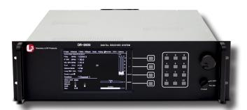
L3 Telemetry & RF Products (L3 T&RF) DR-2000 receiving unit incorporates a high-performance telemetry RF section, a DSP-based multimode demodulator with pre-programmed FIR IF and video filters, and an optional tunable bit synchronizer within a single, 5.25-inch rack-mounted chassis.
